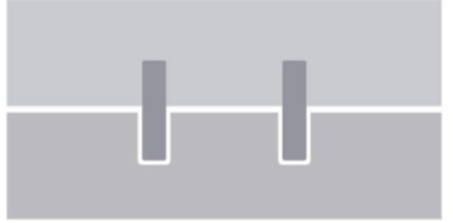
hole and slot with metal pins
