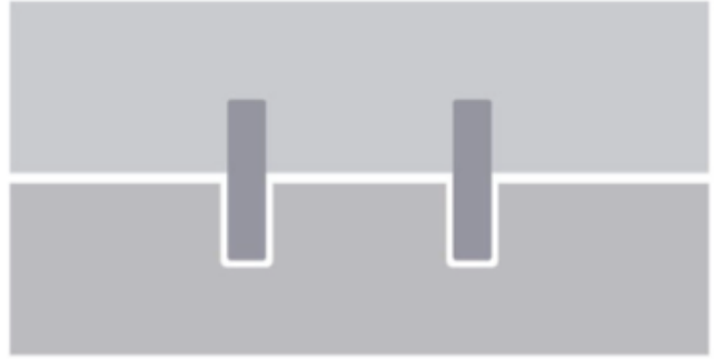
hole and slot with metal pins
